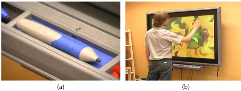
Figure 14: The pen tray (a) is used to switch between a sketching and distribution context. A user gradually fades out strokes with a flat hand in the distribution context (b).
