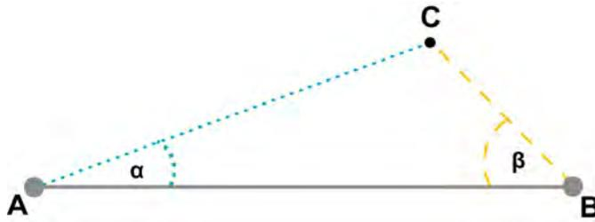
Figure 35: Coordinates of point C can be calculated through triangulation, if the distance  $\overline{AB}$  and the two angles  $\alpha$  and  $\beta$  are known.
