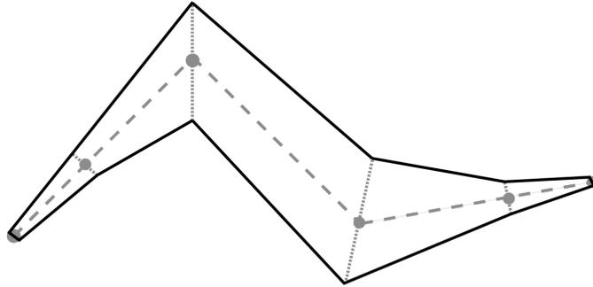
Figure 21: Stroke control points (black dots), vectors between control points (dashed gray lines), bisectors (dotted gray lines), and boundary lines of associated OpenGL quad strip.
