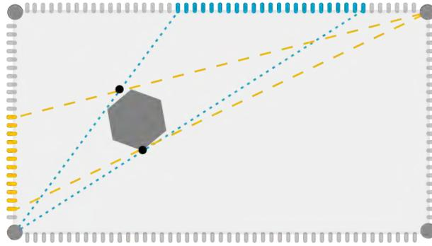
Figure 12: With each camera two angles of an touching object can be recognized. The angles are used for determining the position of object boundary points through triangulation.
