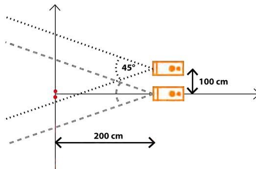
Figure 16: At a pointing distance of 2 meters the maximal lateral displacement is 1 meter if the *Wiimote* is held orthogonal to the screen.
