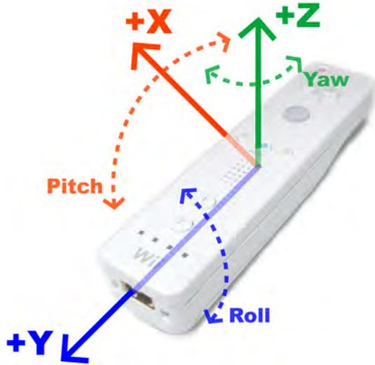
Figure 37: Coordinate system of the *Wiimote*.
