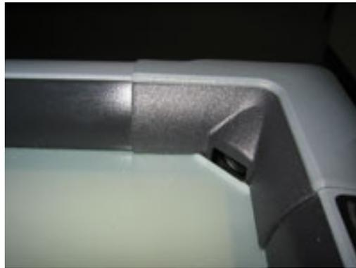
Figure 2.2: Cameras in each corner of the DViT.
