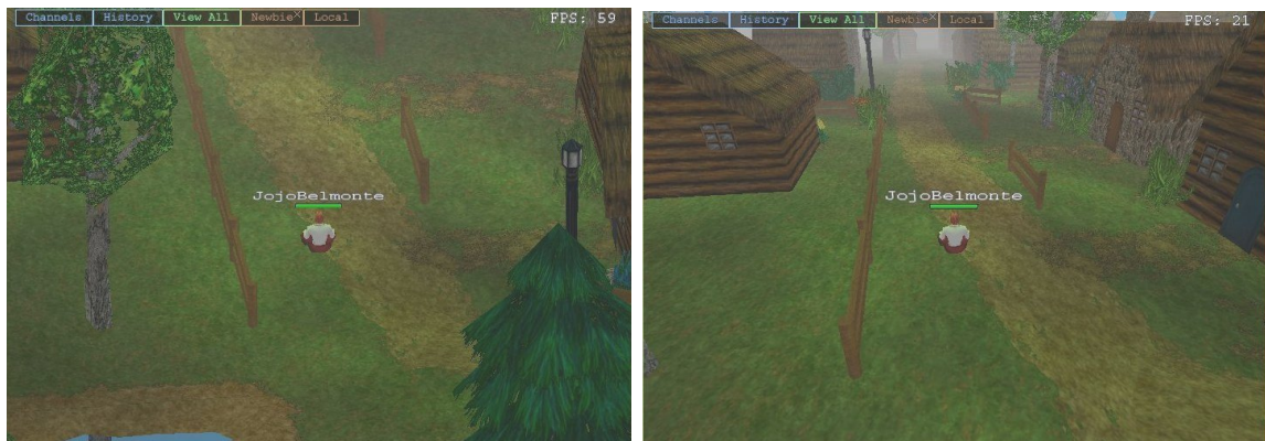
(a) Without perspective projection. Notice how the fences appear parallel (b) With typical perspective projection. Notice how the fences and buildings on each side of the path appear to converge in the distance
