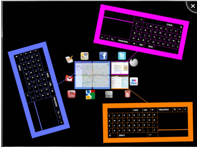
Figure 4. The window manager in the center of the horizontal display shows the wall-display contents (see Figure 3) and is surrounded by an application launcher. Virtual input devices have been opened for controlling each of the three windows.
