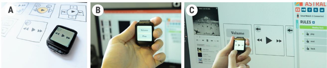
Figure 8. Astral supports the design process in all stages by allowing (a) on-device rapid creation of interactive sketches (Scenario 3A), (b) using slideshows to transition between states (Scenario 3B), or (c) creating interactive images (Scenario 3C).
