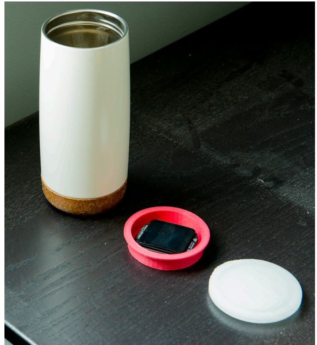
Figure 10. "Smart Home Speaker" prototype (Scenario 5) consisting of a travel mug, a smart watch, a 3D-printed base to hold the watch and a translucent 3D printed lid that diffuses light.
